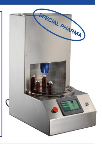
The CR-5000S is versatile, stable, and allows the crimping force to be adjusted precisely. The interchangeable crimping heads are quickly fitted without tools and are especially suited for crimping aluminium and steel caps with diameters of 8, 11, 13, and 20 mm. Special heads are available for 13 mm and 20 mm flip-off caps.
