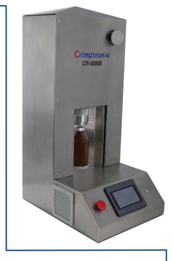
The CR-4000SL is versatile, stable, and allows the crimping and decapping force to be adjusted precisely. The interchangeable crimping or decapping heads are easily fitted without tools and are specially suited for crimping and decapping aluminium and steel caps with diameters of 8, 11, 13, 20, and 32 mm, as well as FEA pumps.
