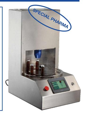
The CR-5000S is versatile, stable, and allows the crimping force to be adjusted precisely. The interchangeable crimping heads are quickly fitted without tools and are especially suited for crimping aluminium and steel caps with diameters of 8, 11, 13, and 20 mm. Special heads are available for 13 mm and 20 mm flip-off caps.
